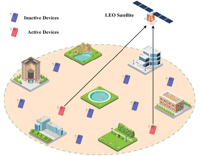
Fig. 1. An illustration of URA system in LEO satellite IoT scenarios.
